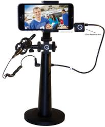
Description: The Que IQ Rig is another option that includes microphone and tripod all in one device. This is good for filming a smaller classroom of students and if you do not have to film a lot of movement. This device is compact and easy to use.
