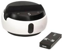
Description: This is a sensor driven robotic platform used with iPod, iPad, or other smartphone for recording. This is extremely efficient if there is a lot of movement involved in a lesson plan. Some other perks of this device is its mobility, compactness, and the use of the marker (sensor) used as a microphone. This allows for improved sound and visibility.
