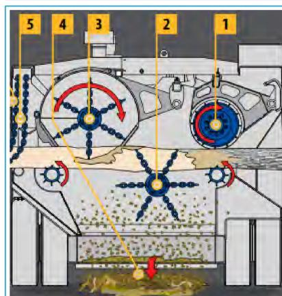
1. Direct drive upper feed feeds the machine 2. Fixed lower chain flail removes the bark from the underside of the stems 3. Floating upper chain flail removes the remainder of the bark from tops & side of the stem 4. Bark & limbs as waste residues 5. Chain curtain sweep
