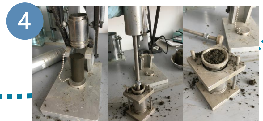
4 Sample Preparation (via modified Harvard Miniature Compaction) and Curing Period
