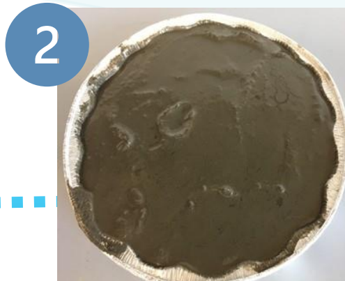
2 Mixture Preparation and "Mellowing" Period
