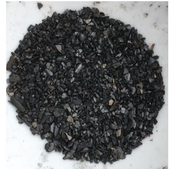
Conowingo Dam sediments contain significant coal deposits (photo from 2021 treatability study conducted by Rutgers and Tipping Point)
