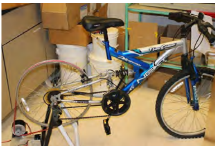
Bike used as generator
