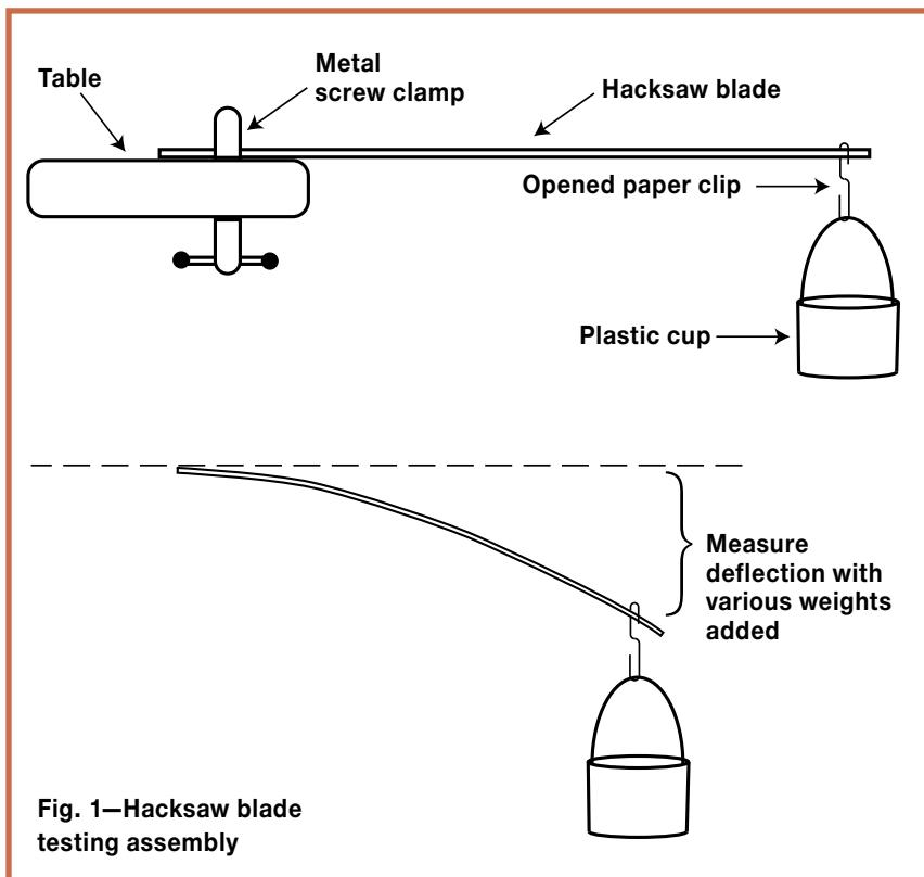
a wire handle added. (See Fig. 2.) The cup is suspended from the saw blade using an opened paper clip that is hooked through a small hole at one end of the saw blade. (Note that a hole is pre-drilled at both ends of the saw blade.)
