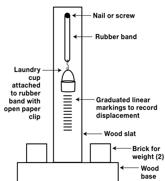
**Fig. 3—Rubber band testing apparatus**
