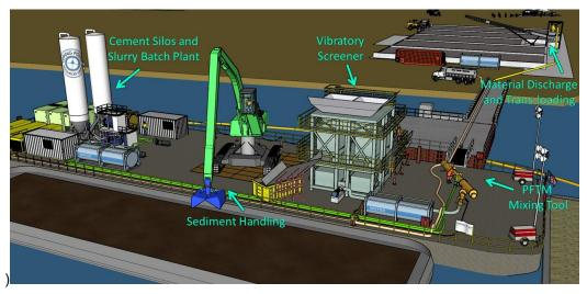
Figure 3-26 Barge-mounted PFTM Operations: Mobile Operating Sediment Engineering System (MOSES)
