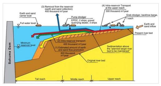
Figure 5-7 Sediment management at the Sakuma Dam (provided by J-Power)
