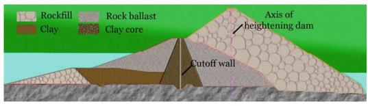
Figure 5-19 The profile of the heightened dam (Yumeng et al., 2020)
