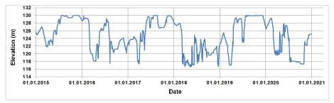
Figure 2-26 Variation of the Channel reservoir level during 2015-2020
