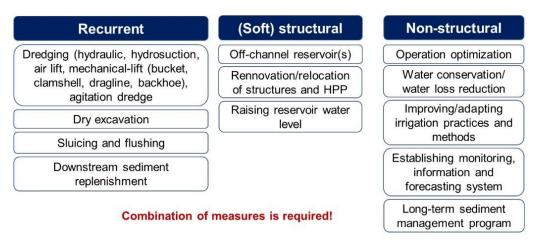
Figure 3-1 Possible measures to manage sediment-induced problems at THC
