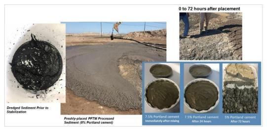
Figure 3-25 Processed sediment using PFTM
