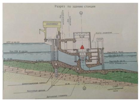
Figure 2-7 A longitudinal profile along the hydropower plant
