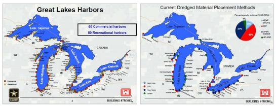
Figure 3-28 Great Lakes harbours (left) and the dredged material placement location and methods (courtesy: D. Romano, 2015)
