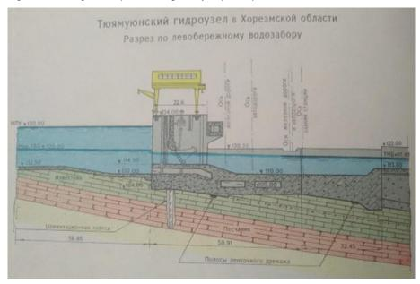
Figure 2-8 A longitudinal profile along the left-bank canal
