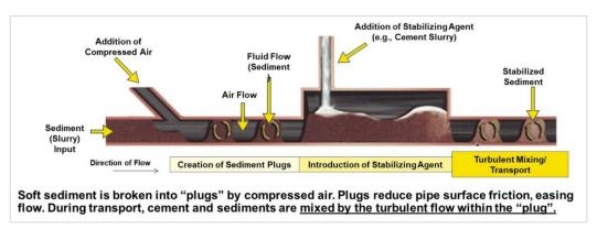
Figure 3-23 PFTM mechanism (Kitazume, 2002)
