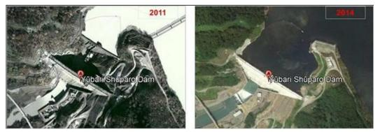
Figure 5-17 Comparing the Google Earth image showing before (left) and after (right) removal of Oyubari dam
