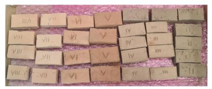
Figure 2-25 The ready sample product (bricks), made using the samples of the Channel reservoir sediment (Central Asian Institute for Ecological Research, 2022)
