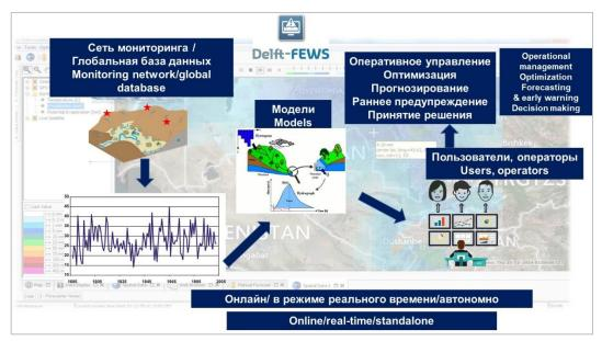
Figure 3-36 Basic principle and components of Delft-FEWS
