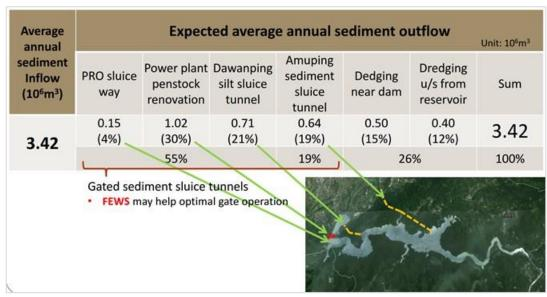
Figure 5-6 Existing and proposed sediment management measures in Shihmen reservoir and expected results of their implementation (Courtesy: Jinn Chuang Yang)
