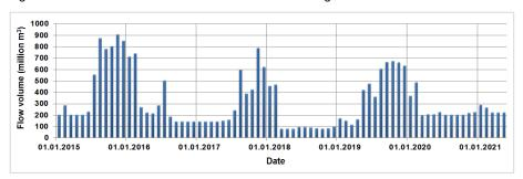
Figure 2-27 Variation of monthly-averaged flow volumes in the Channel reservoir during 2015-2021
