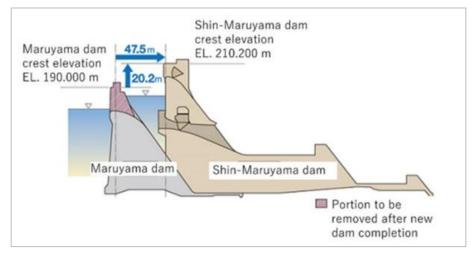
Figure 5-14 Upgrading (heightening) the Maruyama dam
