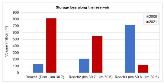
Figure 2-18 Comparing the storage loss along the Channel reservoir between 2008 and 2021
