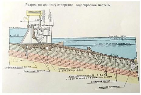
Figure 2-6 A longitudinal section along the undersluices
