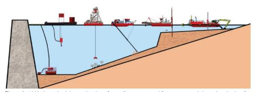
Figure 3-14 Various dredging technology for sediment removal from a reservoir based on hydraulic and morphological condition (provided by Royal IHC)
