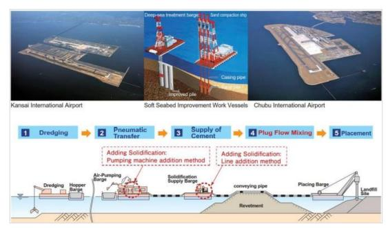
Figure 3-27 Examples of artificial island in Japan (upper images), built using PTFM technique (lower image shows the workflow and features of dredged sediment recycling system (Giri et al., 2019, internet source)
