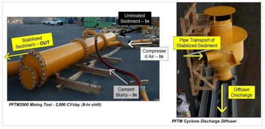
Figure 3-24 PFTM process equipment
