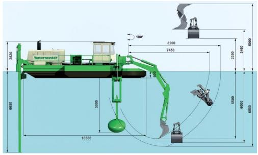
Figure 3-15 Amphibious multipurpose Watermaster – applicable for dry areas to the depth up to 6.5 m; the pumping rate is 600-900 m³/hr (with 10-30% of solids) with max. pumping distance up to 1.5 km. The production rate is very much affected by various conditions, e.g. soil condition, pumping height and distance, presence of debris or stones, operators experience, etc. (https://watermaster.fi).
