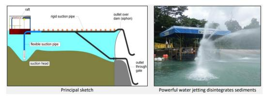
Figure 3-16 The SediCon Dredge is a hydrosuction system that uses the available water head between the reservoir and the outlet of the discharging pipe, for pumping out water and sediments (so, it does not require energy). Typical average capacity range from 50 m³ cohesive sediments per hour for 200 mm dredges and up to 1000 m³ per hour for sandy materials dredged with a 500 mm dredge (<a href="www.sedicon.no">www.sedicon.no</a>).
