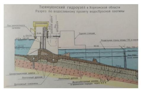
Figure 2-5 A longitudinal section along the spillway
