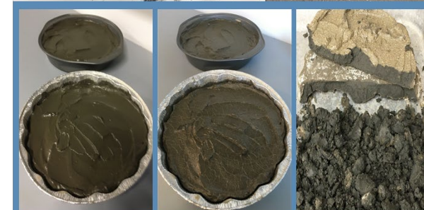
7.5% Portland cement Immediately Post-mixing
