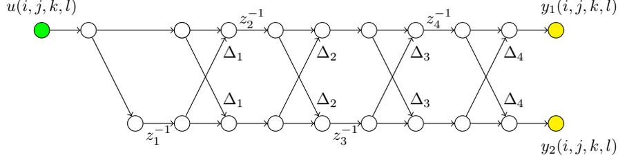
Fig. 2: 4D first-order lattice FIR digital filter with alternate delays.
