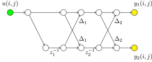
Fig. 5: 2D first-order lattice FIR conventional digital filter.
