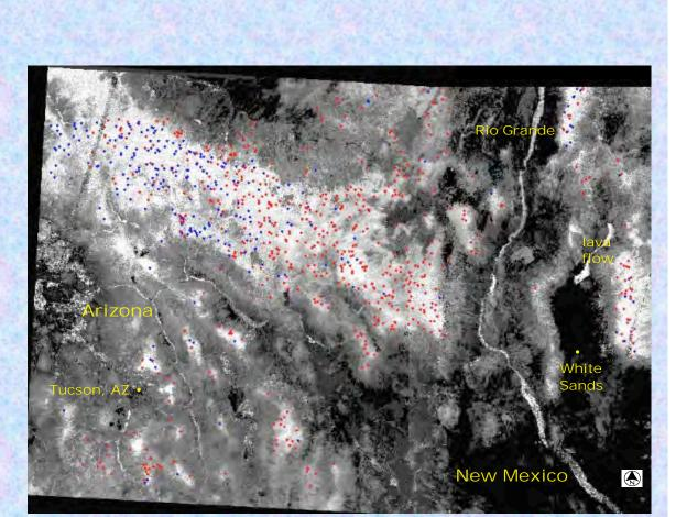
Figure 4. MISR/GO crown cover map in grayscale showing illuminated reference locations (red points) and those impacted by topography (blue points).
