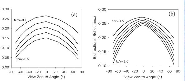
Figure 2. The effects of changing (a) fractional crown cover with plant number density ( $\lambda$ ) fixed at 0.012 and maintaining canopy height at 3.0 m (b) crown shape (b/r), maintaining h/b fixed at a typical value of 2.00, where r, b and h are crown horizontal radius, vertical radius and center height.
